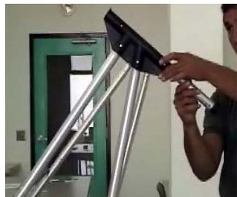
30. Remove **feet** from **legs**. Place in correct location outside of case.
