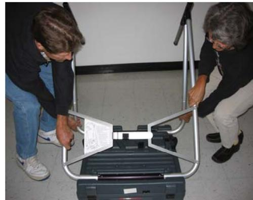
29. Push **foot extenders** in all the way on both sets of legs. Note: Press button to unlock **extender**.
