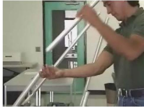
32. Grasp **FRONT leg** while pressing button to release lock; fold down until flat against case. Repeat for other **FRONT Leg**.
