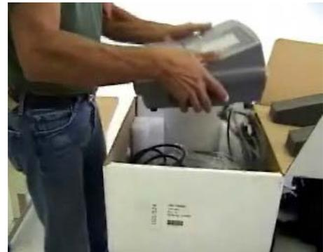
20. Coil the **JBC cable** and **power cord**; place to one side of JBC inside box.
