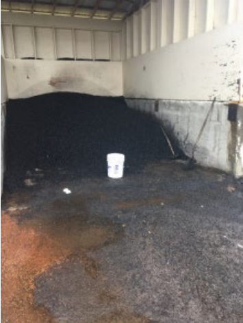
Cold Mix Asphalt Repair Material Shovel and 5 Gallon Bucket for Pot hole repair
