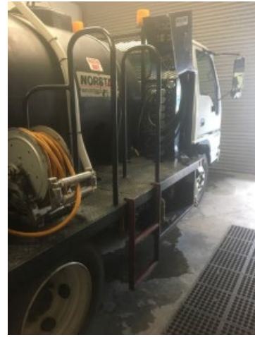
Side of Spray/Tank Truck- Portable Ladder Steps at 12" – 24" – 36" to bed of truck
