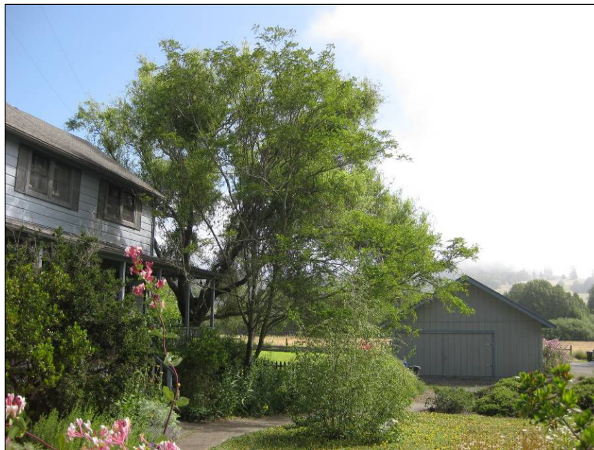
Figure 37: Residence, 489 Bohemian Highway. The new detached garage (on the right) is located away from the historic residence (on the left) at an appropriate distance. The garage's one-story height, gabled roof, wood siding, and paint color do not detract from the historic house.
