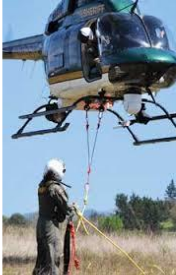
Figure 2: Cable Attachment to Helicopter
